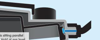
Ensure the silicone is sitting parallel on the hole below it. Hold at eve level to check the position is correct
